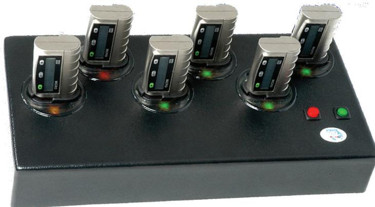
Once the test has been completed (red or green LED), remove the detectors and replace them with additional units. Additional detectors can only be tested if checked units have been removed.
