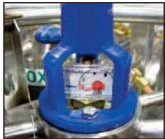
The Roto-Tel™ Liquid Level Gauge offers improved accuracy and expanded gauge ranges for better resolution.
